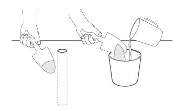
4 Place sensor in vertical position (do not tilt more than 45°) at bottom of hole.
