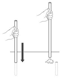
3 Mix a slurry of native soil and water. Pour the mixture into the hole.
