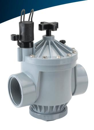
The Irritrol® 200B Series globe/angle valves have built their popularity on a proven record of reliability and a reputation for offering valuable features at an affordable price. The 200B Series provides manual internal and external bleed, heavy-duty, UV-resistant PVC construction, stainless steel hardware, a double-beaded diaphragm and a captive solenoid plunger.
